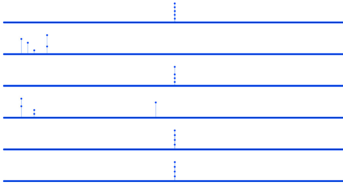
Fig. 9 Ranking of top five nodes in 6-regular (Test 2 in Table 2, |V| = 10^6 ) by the comparison algorithms. Horizontal axes show the node indices from 1 to |V| . Marker heights correspond to the rankings of the nodes (higher marker indicates higher ranking). From top to bottom , the six plots show the rankings given by potential values, and the five comparison algorithms: Metropolis–Hastings (MH), global Metropolis–Hastings (GMH), random walk only (RW), random teleportation (RT) only, combination of random walk and teleportation (RWT)
